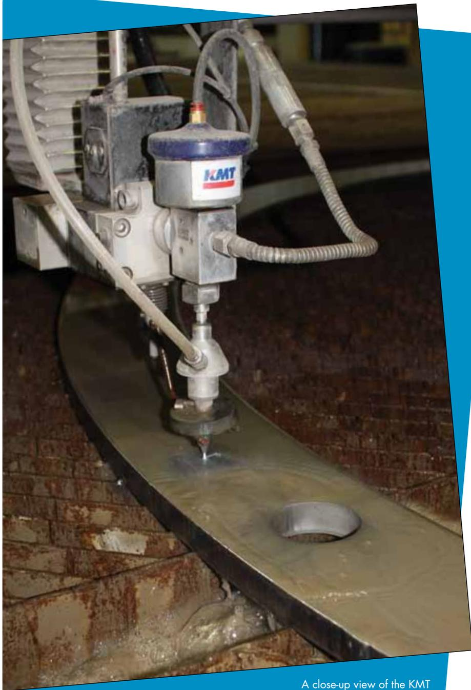
A close-up view of the KMT waterjet cutting head.
