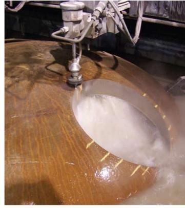
clad w/~1/4" of Inconel Alloy 625. Because all work was done in reference to the vessel's axis actual cutting thickness ranged from 3-1/8" to 6".
