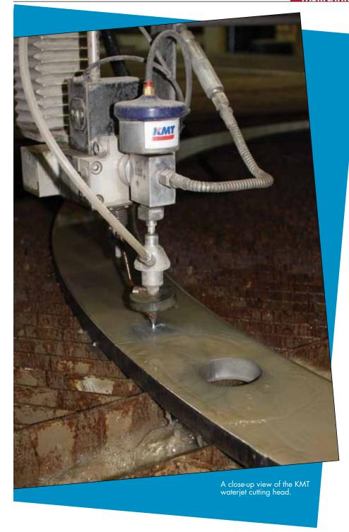
Powering the Zuccatos' machine shop is the zippy KMT Waterjet cutting system. Paul points out that KMT supplied the intensifier, all high pressure lines from the intensifier to the cutting heads, high pressure fittings, cutting heads, mini feeders, and large garnet hopper. Advanced Profiles has incorporated the KMT equipment with the gantry, cutting table and garnet removal system made by ESAB, welding consumables and
