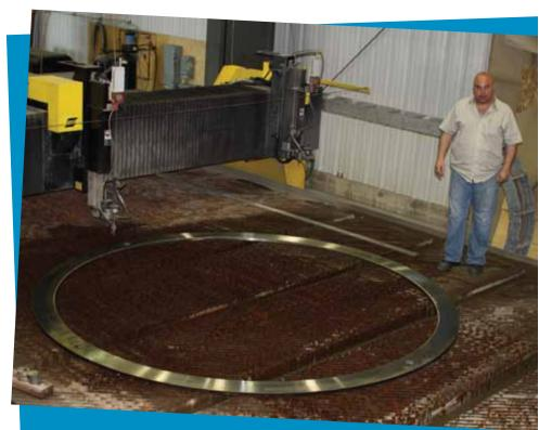
The KMT waterjet is equipped with what Dennis Zuccato says is one of the industry's largest cutting tables, stretching 18 ft (5.5 m) wide by 37 ft (11.3 m) long, with clearances of 13 in. (table to torch), 17-3/8 in. (table to gantry) and 23-3/8 in. (base to gantry).
